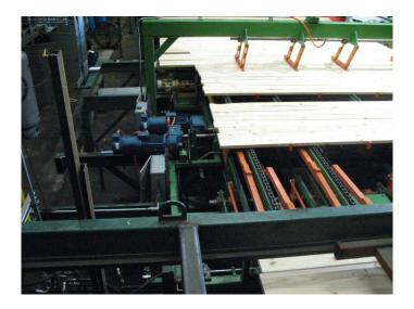
The Dual Fork Stacking arms are raised and lowered with crank arms on shafts, powered by Electric positioners. Hydraulic positioners could also be used in this area if hydraulic systems are available. The hydraulic positioners require about 22 GPM at 2000 psi to run at 24 cycles per minute.
