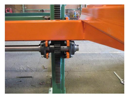
Eccentric Bushings allow the lifts to be level front to back
