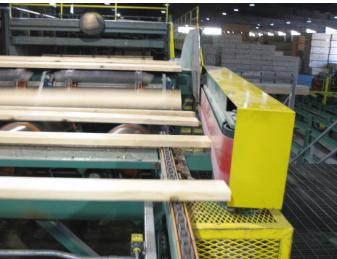
The incline chains, unscrambler, spiral rolls, belt even ender, and infeed chains are individually driven with VFD's for optimum performance.
