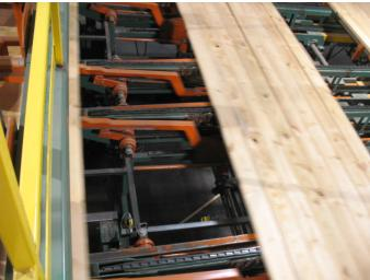
The Dual Fork Stacking arms ride on bearing sled assemblies with yoke style cam followers. The bearings ride on AR plate, and the arms are powered back and forth by a rack and pinion system.
