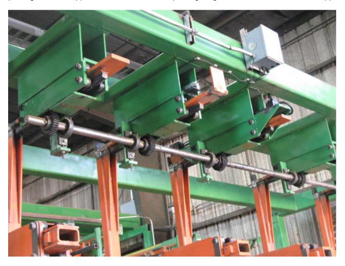
The 4' long vertical arms are used to crowd each course as it is placed on the package being formulated as well as also used to compress the completed package for the automatic application of the package retaining hoop in order to hold the package together as it is lowered and transported to the strapper.
