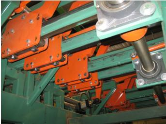
The Dual Fork Stacking Arms are set to cycle up to 26 CPM whenever a completed course of lumber is in position to be stacked. This will net about 22 layers per minute when stacking dimension sizes. There are 5 speed levels and are automatically or manually set depending on the product size.
