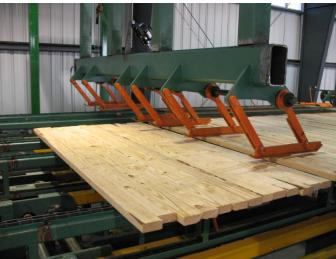
The lower course pinch off is unique in that it not only pinches off the course of lumber to be stacked, but raises up to block the incoming layer of lumber against the face of the pinch off arm so that lumber can't push its way through the pinch off.
