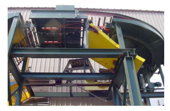
Once the stickers pass the quality control scanning section, they are fed to the pusher lug distribution chains where they are loaded into the sticker storage magazines.
