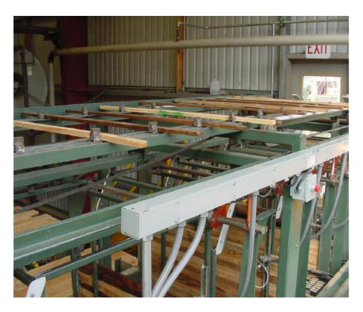
While the above automatic sticker loading system will eliminate the need for an operator, the sticker storage magazines may also be loaded manually.
