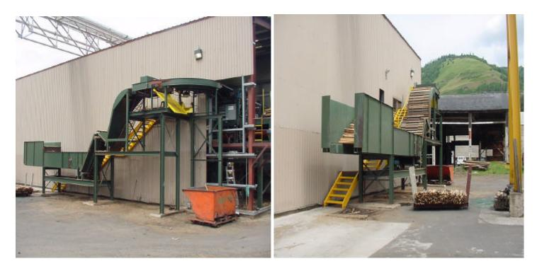
Loose bundles of stickers are placed into the bulk chains of the automatic infeed.
